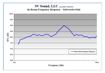
To correct a peak such as that above, start by setting the Frequency to about 40 Hz, the Q to HI, and the Level to MAX. Re-measure and re-plot from 30-70 Hz to evaluate the effect.
